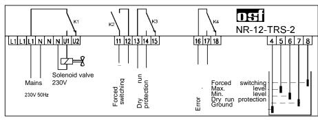
Relay K2 switches the filter pump on once the water level reaches the top electrode.
