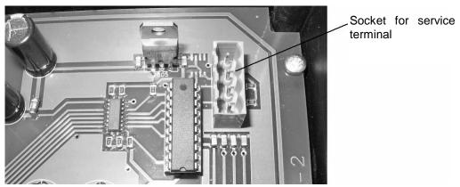
The service terminal is used to display the level regulation operating status clearly in order to help in possible troubleshooting. Caution! The service terminal may only be plugged in or unplugged when the control system is switched off!
