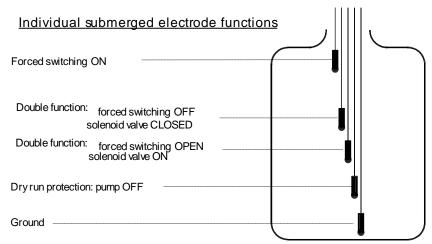
In normal operation, the water level varies between the "solenoid valve CLOSED" and "solenoid valve OPEN".
